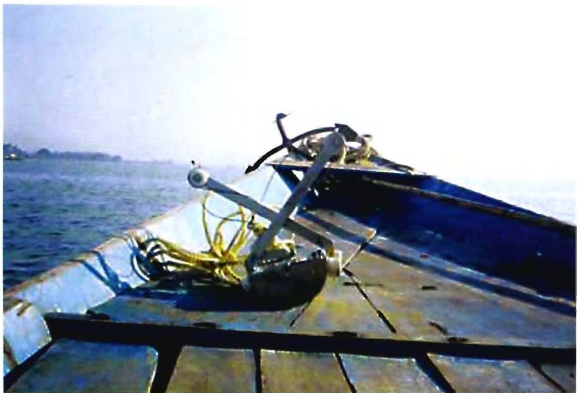
Plate 6. A view of the Peterson's grab (.025 m 2 ) used for benthic collection during the study period.
